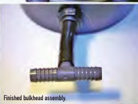
Cut 3/4" vinyl for T assembly and connection.
